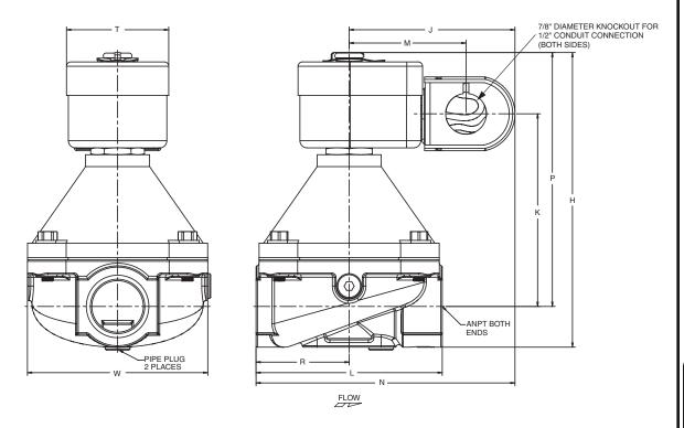
Must be mounted with solenoid vertical and upright or in the horizontal position.
